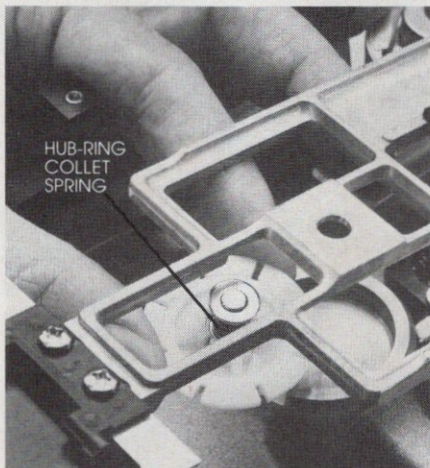
Figure 9: The hub-ring collet clamps the diskette down when the disk-drive door is closed. If the ring does not clamp down securely, look for a weak clamping action due to a defective spring.
