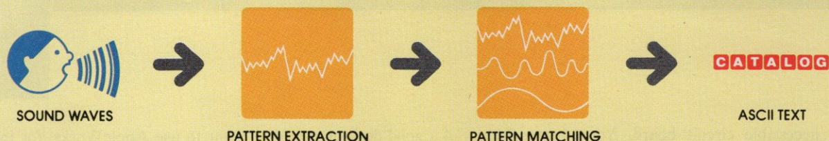
Figure 1: Speech-recognition boards extract patterns from sound-wave inputs, match the patterns against stored templates, and produce characters equivalent to the keystrokes that correspond to the word or phrase best matching the sound-wave inputs.
