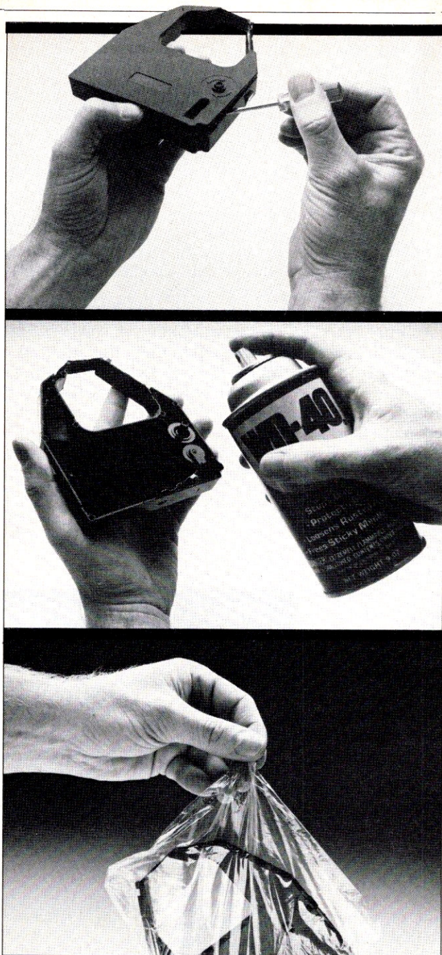
Fig. 2 Solvents can redistribute the ink on a used ribbon. Pry open the cartridge with a screwdriver, spray the ribbon with WD-40 or alcohol, and let it stand in a plastic bag for several days to allow the ink to spread evenly.
