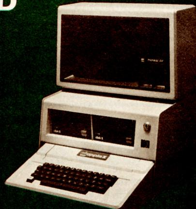
opens up to allow quick and easy access inside your Apple. The key switches power to your Apple system and the filtered cooling fan. The SURGE SENTRY, by RKS Industries, protects your Apple from harmful voltage spikes.
