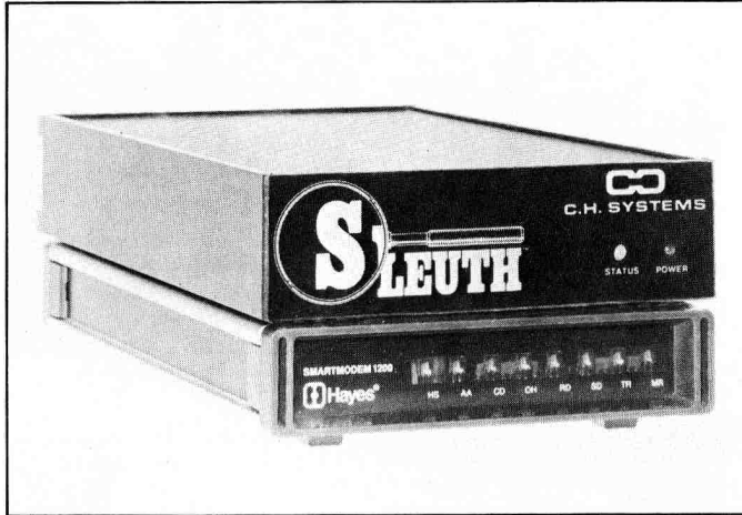
Modem security with the dial-back Sleuth.
