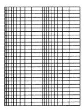
Figure 3. Three-cycle semi-log strip chart.
