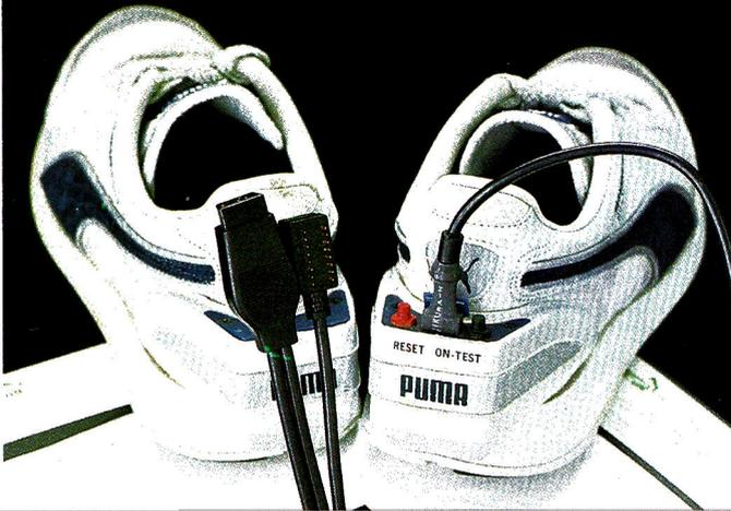
The Puma RS-Computer Shoe looks like a traditional running shoe—with a bad case of heel spurs. A compartment is built into the right heel and houses a compact battery-powered circuit board that functions like a pedometer. Black "On-Test" and red "Reset" buttons protrude from the compartment. A tiny plastic lid protects a recessed four-pin interface port.
