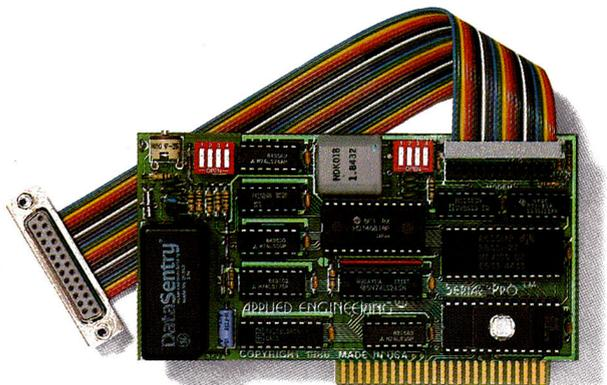
**Serial Pro** is a powerful multifunction card for the Apple IIe, II+, IIGs and compatible computers. Serial Pro combines a powerful serial port for interfacing to a printer, modem or other serial device, with a full function clock/calendar. Serial Pro's serial port is compatible with virtually all letter quality and dot matrix printers, including Apple's Imagewriter and Imagewriter II, and can communicate with the fastest external modems at baud rates from 50 to 19,200.
